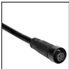
IP67 Connector 4PIN Order Code : 8911616-05 Wire gauge : 0.326mm 2 /22AWG Protection : IP67 (Mated) Connector type : Female
