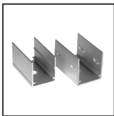
Mounting Clips Order Code : 8911616-03 Dimension : L20xW16.6xH12.4mm Material : stainless steel Color : silver Each meter led strips needs 2 clips + 2 screws
