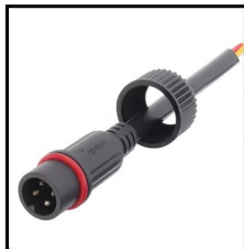
IP67 Connector 4PIN Order Code: 8911515-04 Wire gauge: 0.326mm 2 /22AWG Protection: IP67 (Mated) Connector type : Male
