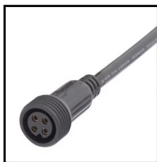
IP67 Connector 4PIN Order Code: 8911212-05 Wire gauge: 0.326mm 2 /22AWG Protection: IP67 (Mated) Connector type : Female
