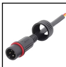
IP67 Connector 4PIN Order Code: 8911212-04 Wire gauge: 0.326mm 2 /22AWG Protection: IP67 (Mated) Connector type : Male
