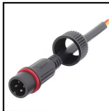
IP67 Connector 4PIN Order Code: 8911010-04 Wire gauge: 0.326mm 2 /22AWG Protection: IP67 (Mated) Connector type : Male
