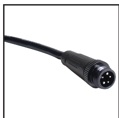
IP67 Connector 5PIN Order Code : 8921616-04 Wire gauge : 0.326mm 2 /22AWG Protection : IP67 (Mated) Connector type : Male
