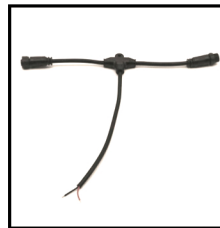
IP67 T Type Connector Order Code: 8921515-08 Wire Gauge: 0.326mm 2 /22AWG Protection: IP67 (Mated)
