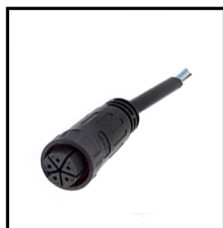
IP67 Connector 5PIN Order Code: 8921010-05 Wire gauge: 0.326mm 2 /22AWG Protection: IP67 (Mated)
