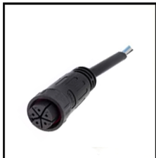
IP67 Connector 5PIN Order Code: 8961818-05 Wire gauge: 0.326mm 2 /22AWG Protection: IP67 (Mated)
