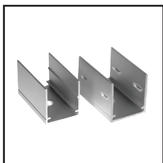
Mounting Clips Order Code : 8961616-03 Dimension : L30xW18xH19mm Material : Stainless steel Color : Silver Each meter led strips needs 2 clips + 2 screws
