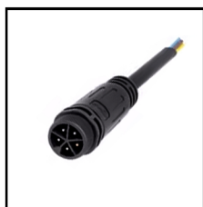
IP67 Connector 5PIN Order Code: 8961212-04 Wire gauge: 0.326mm 2 /22AWG Protection: IP67 (Mated)
