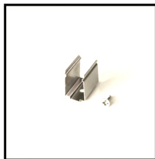
Mounting Clips Order Code: 8961010-03 Dimension: L11.6xW8xH7.6mm Material: stainless steel Color: silver Each meter led strips needs 2 clips + 2 screws
