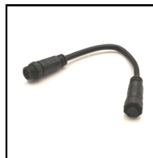
IP67 Signal Connector Order Code: 8961010-10 Wire Gauge: 0.326mm 2 /22AWG Protection: IP67 (Mated)
