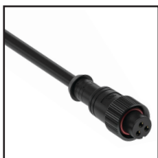
IP67 Connector 3PIN Order Code : 8971616-05 Wire gauge : 0.326mm 2 /22AWG Protection : IP67 (Mated) Connector type : Female
