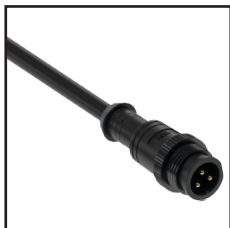
IP67 Connector 3PIN Order Code : 8971616-04 Wire gauge : 0.326mm 2 /22AWG Protection : IP67 (Mated) Connector type : Male
