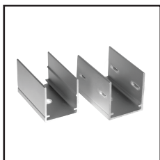
Mounting Clips Order Code : 8971616-03 Dimension : L30xW16.9xH17.8mm Material : stainless steel Color : silver Each meter led strips needs 2 clips + 2 screws
