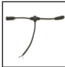
IP67 T Type Connector Order Code: 8971310-08 Wire Gauge: 0.326mm 2 /22AWG Protection: IP67 (Mated)
