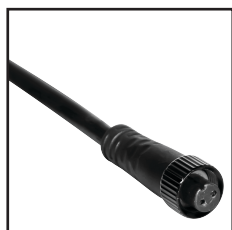
IP67 Connector 2PIN Order Code : 8982010-05 Wire gauge : 0.326mm 2 /22AWG Protection : IP67 (Mated) Connector type : Female
