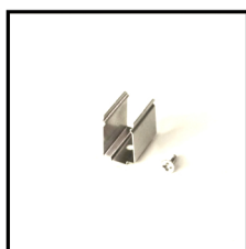
Mounting Clips Order Code: 8931818-03 Dimension: L30xW19.8H16.9 Material: stainless steel Color: silver Each meter led strips needs 2 clips + 2 screws
