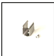
Mounting Clips Order Code: 8931818-03 Dimension: L30xW19.8H16.9 Material: stainless steel Color: silver Each meter led strips needs 2 clips + 2 screws
