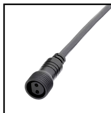
IP67 Connector 2PIN Order Code: 8931818-05 Wire gauge: 0.326mm 2 /22AWG Protection: IP67 (Mated)
