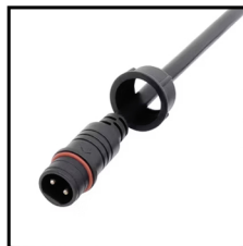
IP67 Connector 2PIN Order Code: 8981616-04 Wire gauge: 0.326mm 2 /22AWG Protection: IP67 (Mated)
