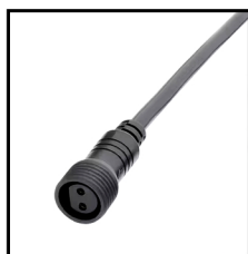
IP67 Connector 2PIN Order Code: 8981616-05 Wire gauge: 0.326mm 2 /22AWG Protection: IP67 (Mated)
