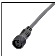
IP67 Connector 2PIN Order Code: 8981515-05 Wire gauge: 0.326mm 2 /22AWG Protection: IP67 (Mated)
