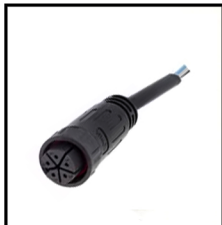
IP67 Connector 5PIN Order Code: 8991818-05 Wire gauge: 0.326mm 2 /22AWG Protection: IP67 (Mated)
