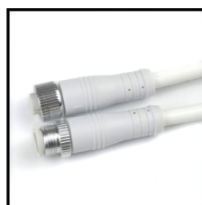
IP67 Connector 2PIN Digital Order Code: 8981212-04 Wire gauge: 0.326mm 2 /22AWG Protection: IP67 (Mated)
