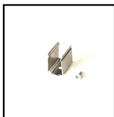
Mounting Clips Order Code: 8941212-03 Dimension: L11.6xW14xH14.6mm Material: stainless steel Color: silver Each meter led strips needs 2 clips + 2 screws
